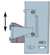
Check if the door opens and closes without hitting the bracket.
