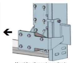
Mount the other part according to picture using supplied bolts and nuts.
