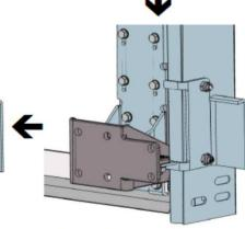
Use supplied track bolts (2x) and nuts (2x) to mount the bracket.
